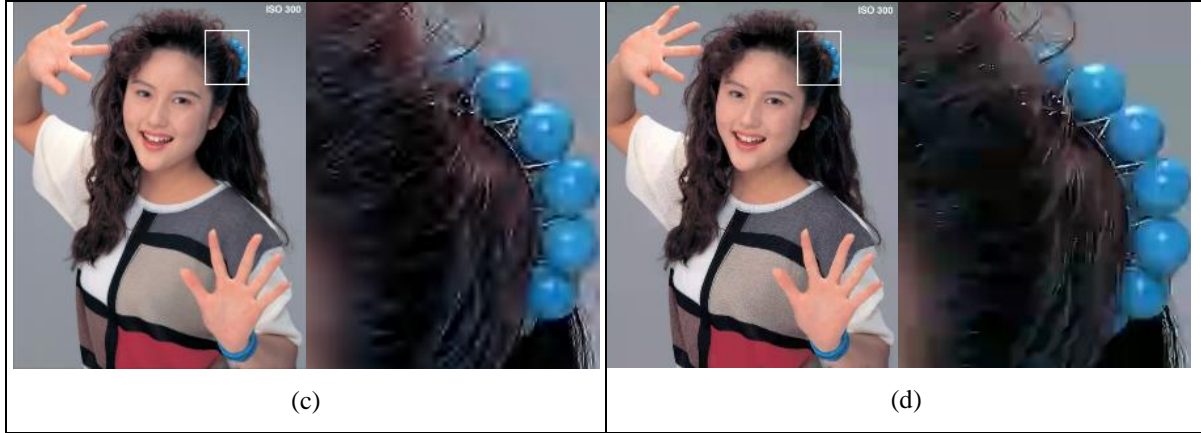
Figure 2. An image and its blurred versions (left), and partially magnified images (right): (a). original image, (b). Gaussian low-pass filtered, (c). JPEG2000 compressed, and (d). H.264 compressed
